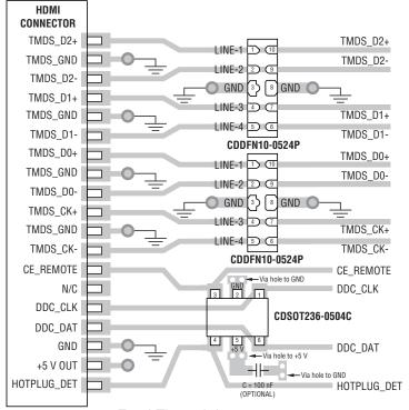
Feed-Through Layout -Model CDDFN10-0524P in HDMI Application
