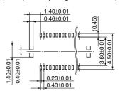
Recommended metal mask pattern Metal mask thickness: Here, 120 μm (Terminal portion opening area ratio: 66%) (Metal portion opening area ratio: 100%)
