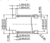
Recommended metal mask pattern Metal mask thickness: Here, 120 μm (Terminal portion opening area ratio: 66%) (Metal portion opening area ratio: 100%)
