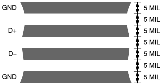
Figure 21. Typical Arrangement of Signal Tracks
