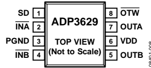
Figure 7. ADP3629 Pin Configuration
