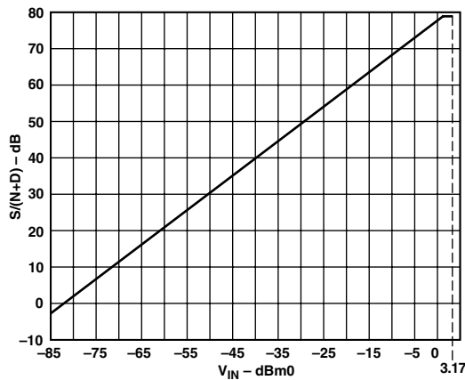
Figure 5d. S/(N+D) vs. V_{IN} (DAC @ 5 V) over Voiceband Bandwidth (300 Hz – 3.4 kHz)
