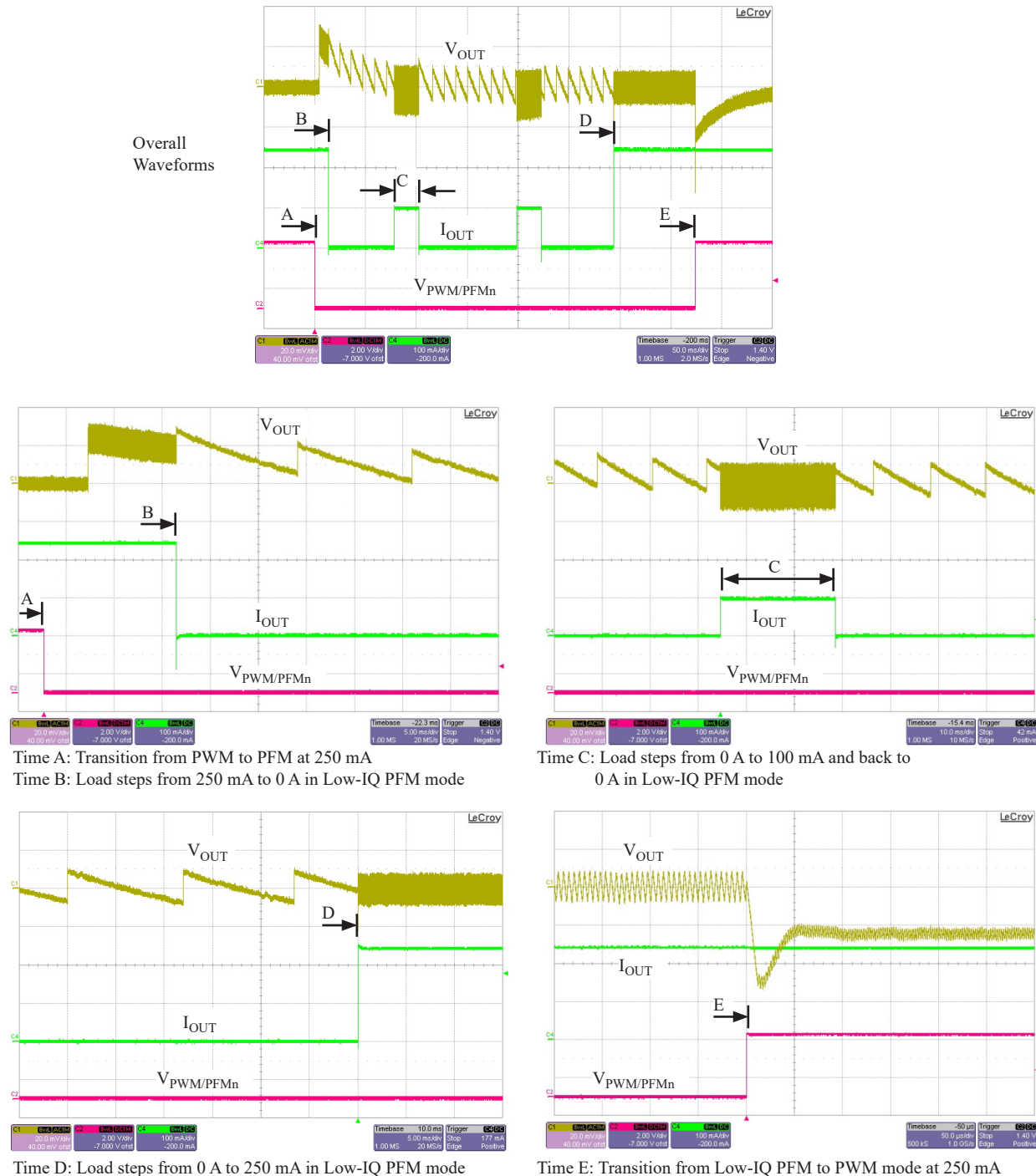
Figure 6: Transitions between PWM Mode and Low-IQ PFM Mode, and Load Transient Responses; using circuit in typical application schematic B ( V_{IN} = 12\text{ V} , V_{OUT} = 5\text{ V} , f_{SW} = 425\text{ kHz} )
