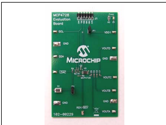
FIGURE 8-1: MCP4728 Evaluation Board.
