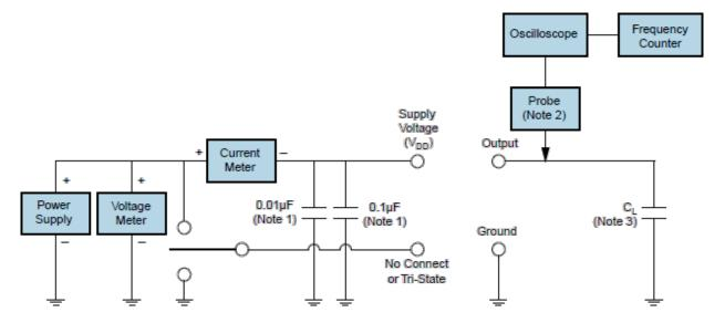
Note 1: An external 0.1μF low frequency tantalum bypass capacitor in parallel with a 0.01μF high frequency ceramic bypass Capacitor close to the package ground pin is required.
