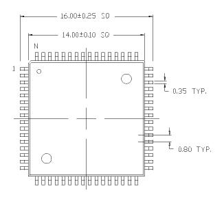
DIMENSIONS IN MILLIMETERS LEAD COPLANARITY 0.102 MAX.
