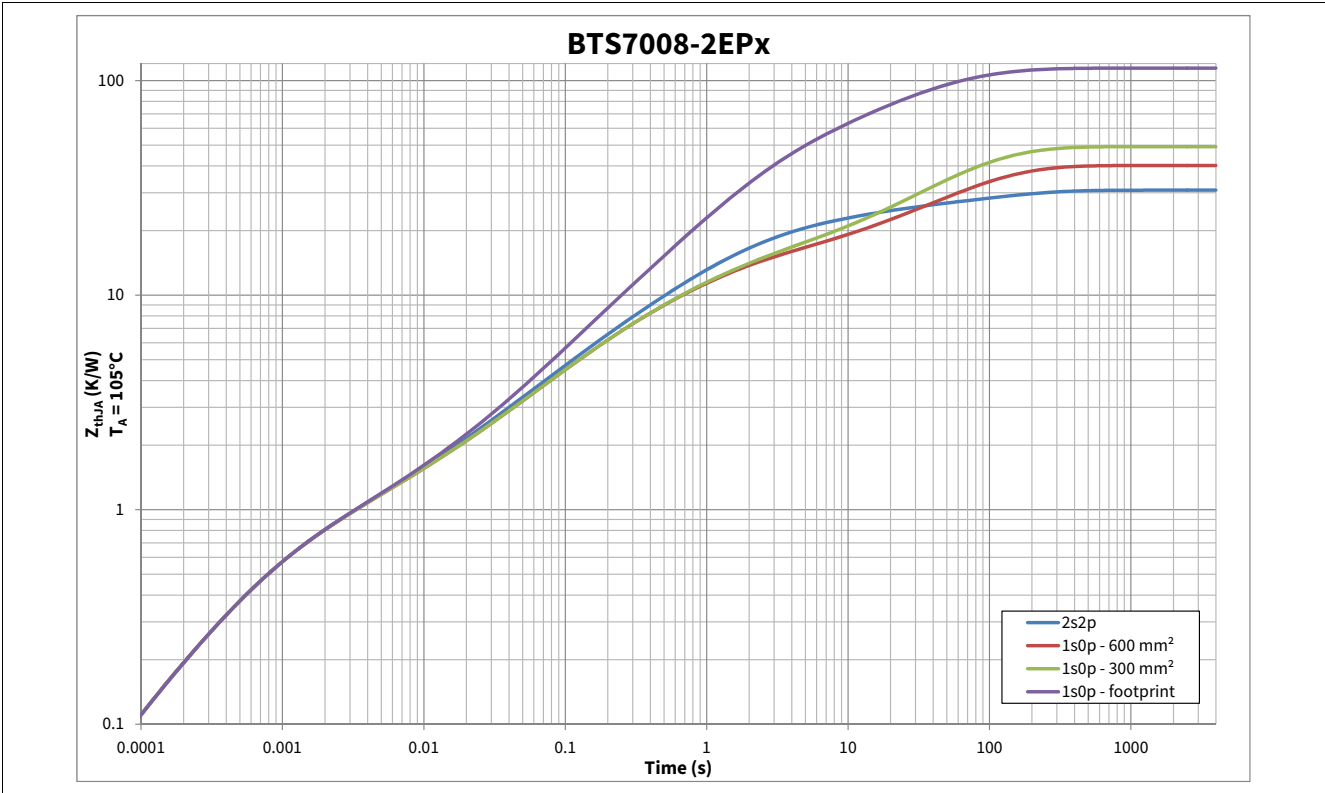
Figure 9 Typical Thermal Impedance. PCB setup according Chapter 4.4.1
