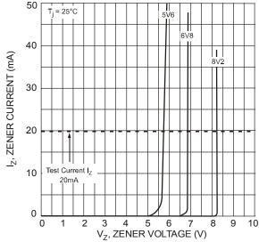
Fig. 2 Typical Zener Breakdown Characteristics
