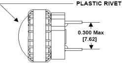
Terminal Dimensions Customer to determine PCB pad dimensions.
