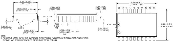
\*DIMENSION DOES NOT INCLUDE MOLD FLASH. MOLD FLASH SHALL NOT EXCEED 0.006" (0.152mm) PER SIDE
