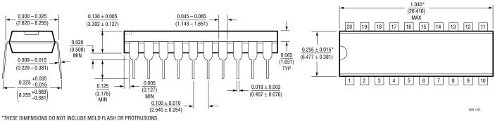
\*THESE DIMENSIONS DO NOT INCLUDE MOLD FLASH OR PROTRUSIONS. MOLD FLASH OR PROTRUSIONS SHALL NOT EXCEED 0.010 INCH (0.254mm)
