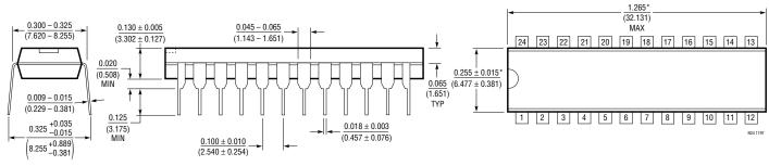
\*THESE DIMENSIONS DO NOT INCLUDE MOLD FLASH OR PROTRUSIONS. MOLD FLASH OR PROTRUSIONS SHALL NOT EXCEED 0.010 INCH (0.254mm)
