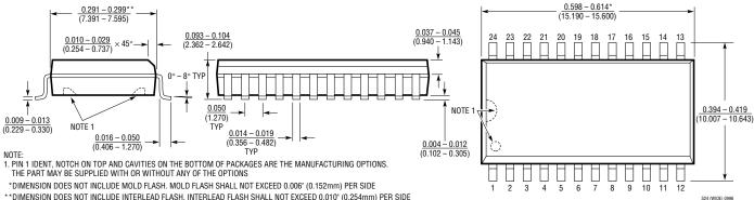
\*\*DIMENSION DOES NOT INCLUDE INTERLEAD FLASH. INTERLEAD FLASH SHALL NOT EXCEED 0.010" (0.254mm) PER SIDE
