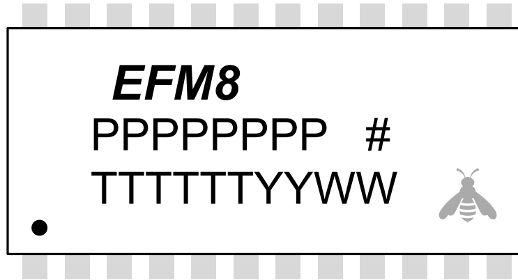
Figure 7.3. QSOP24 Package Marking
