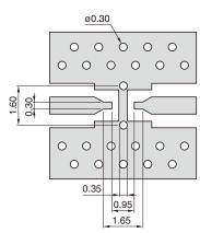
Line width be designed to match  $50\Omega$  characteristic impedance depending on PCB material and thickness.
