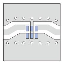
Line width to be designed to match  $50\Omega$  characteristic impedance, depending on PCB material and thickness.
