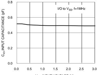
$\label{eq:V_I/O_INPUT VOLTAGE} V_{I/O_i} \mbox{INPUT VOLTAGE (V)} \\ \mbox{Figure 2. Input Capacitance vs. Input Voltage}$
