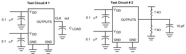
For parameter t<sub>8</sub> (output slew rate) on -1H devices
