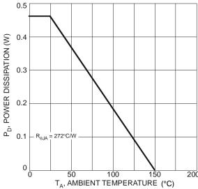
Fig. 3 Power Dissipation vs. Ambient Temperature
