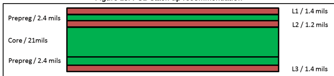
Figure 18: PCB stack-up recommendation
