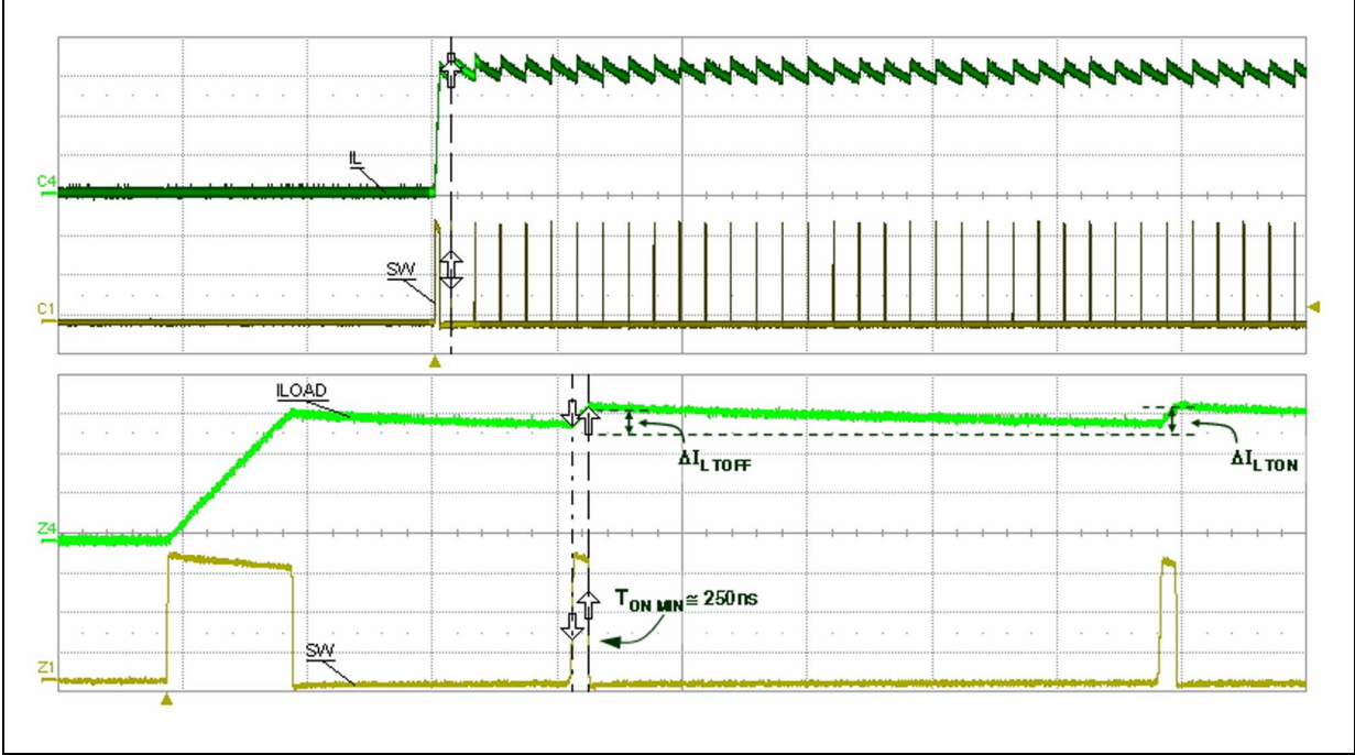
Figure 16. Short-circuit current V_{IN} = 24\text{ V}
