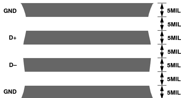
Figure 21. Typical Arrangement of Signal Tracks
