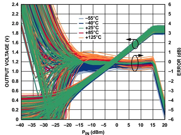
Figure 26. Distribution of Log Conformance Error with Respect to Calibration at 25°C vs. Input Level and Temperature at 2.6 GHz
