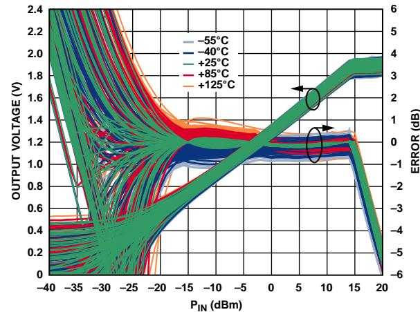
Figure 25. Distribution of Log Conformance Error with Respect to Calibration at 25°C vs. Input Level and Temperature at 2.14 GHz
