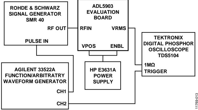
Figure 36. Hardware Configuration for Output Response to RF Burst Input Measurements
