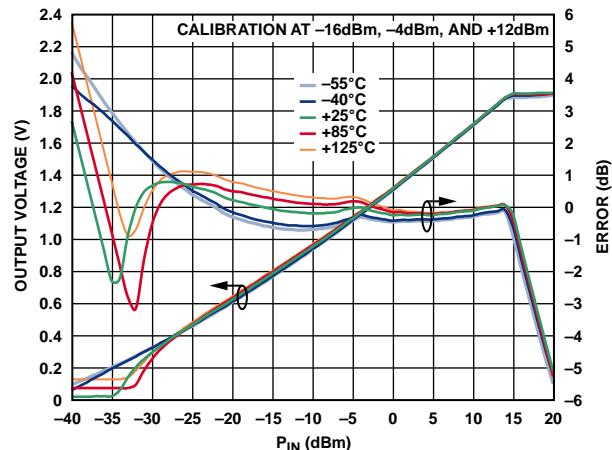
Figure 47. 2.14 GHz  $V_{RMS}$  and Log Conformance Error for Second Device at  $+25^{\circ}\text{C}$ ,  $-40^{\circ}\text{C}$ ,  $-55^{\circ}\text{C}$ ,  $+85^{\circ}\text{C}$ , and  $+125^{\circ}\text{C}$
