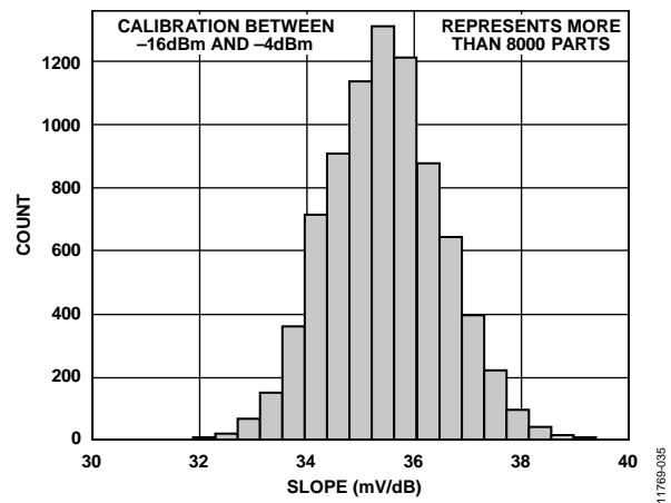
Figure 35. Distribution of Slope at 900 MHz
