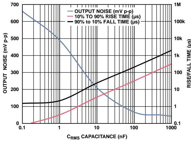
Figure 42. Output Noise, Rise/Fall Times vs.  $C_{RMS}$  Capacitance, Single Carrier W-CDMA (Test Model TM1-64) at 2.14 GHz with  $P_{IN} = 0$  dBm
