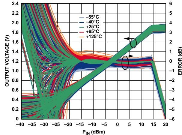
Figure 24. Distribution of Log Conformance Error with Respect to Calibration at 25°C vs. Input Level and Temperature at 1.9 GHz
