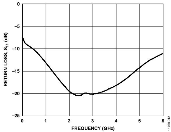
Figure 12. Input Return Loss vs. RF Frequency
