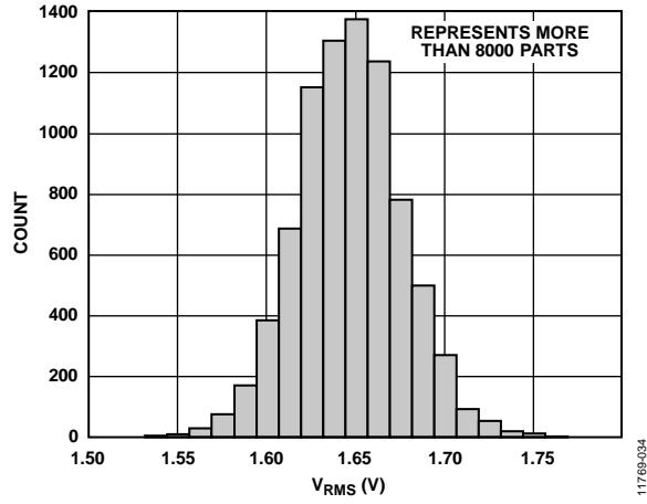
Figure 29. Distribution of  $V_{RMS}$ ,  $P_{IN} = 8 \text{ dBm}$ , 900 MHz
