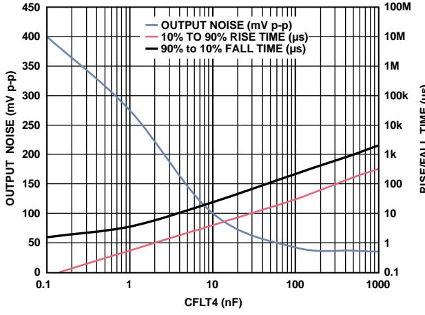
Figure 43. Output Noise, Rise/Fall Times vs.  $C_{RMS}$  Capacitance, Single Carrier LTE (Test Model TM1-20) at 2.14 GHz with  $P_{IN} = 0 \text{ dBm}$
