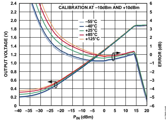
Figure 45. 2.14 GHz  $V_{RMS}$  and Log Conformance Error at  $+25^{\circ}\text{C}$ ,  $-40^{\circ}\text{C}$ ,  $-55^{\circ}\text{C}$ ,  $+85^{\circ}\text{C}$ , and  $+125^{\circ}\text{C}$
