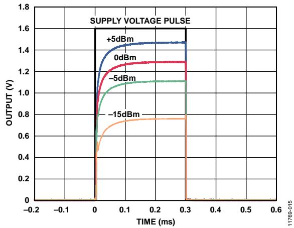
Figure 14. Output Response to Gating on Power Supply for Various RF Input Levels, Carrier Frequency = 900 MHz,  $C_{RMS} = 100 \text{ nF}$ , 5.0 V Supply (see Figure 37, in the Measurement Setups Section))
