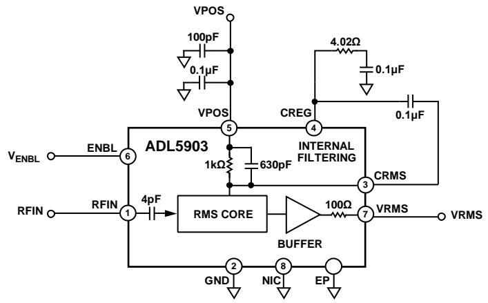
*Figure 44. Basic Connections*
