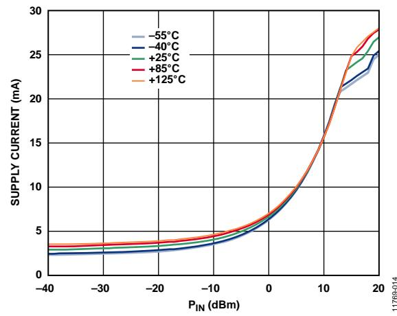
Figure 34. Supply Current vs. Input Level
