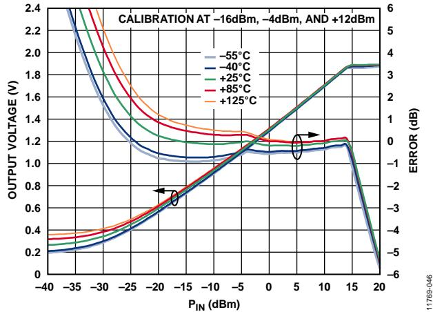
Figure 46. 2.14 GHz  $V_{RMS}$  and Log Conformance Error at  $+25^{\circ}\text{C}$ ,  $-40^{\circ}\text{C}$ ,  $-55^{\circ}\text{C}$ ,  $+85^{\circ}\text{C}$ , and  $+125^{\circ}\text{C}$
