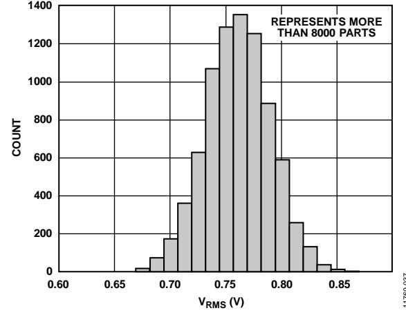
Figure 32. Distribution of  $V_{RMS}$ ,  $P_{IN} = -16 \text{ dBm}$ , 900 MHz
