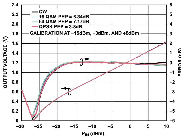
Figure 7. Error from CW Linear Reference vs. Input Level and Signal Modulation (QPSK, 16 QAM, 64 QAM), Frequency = 2.14 GHz, CRMS = 1 μF
