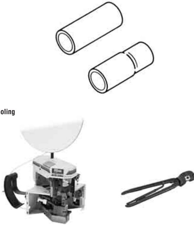
AMP-O-LECTRIC Model "G" Terminating Machine
