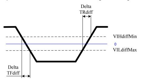
**AC and DC Output Measurement Levels**
