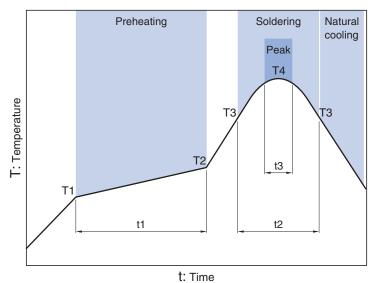
Preheating Soldering Peak Temp. Time Time Temp. Temp. Time T1 T2 t1 Т3 t2 **T**4 t3 150°C 180°C 90 to 120s 230°C 40s 255°C 10s max.
