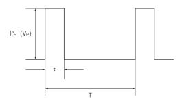
: Pulse limit power (W) : Pulse limit voltage (V) : Pulse continuous time (s)
