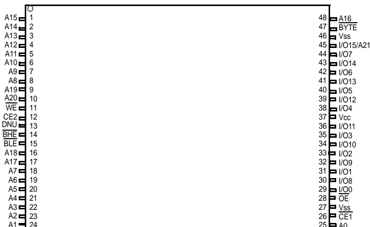
Figure 1. 48-pin TSOP I pinout (Front View) [1, 2]
