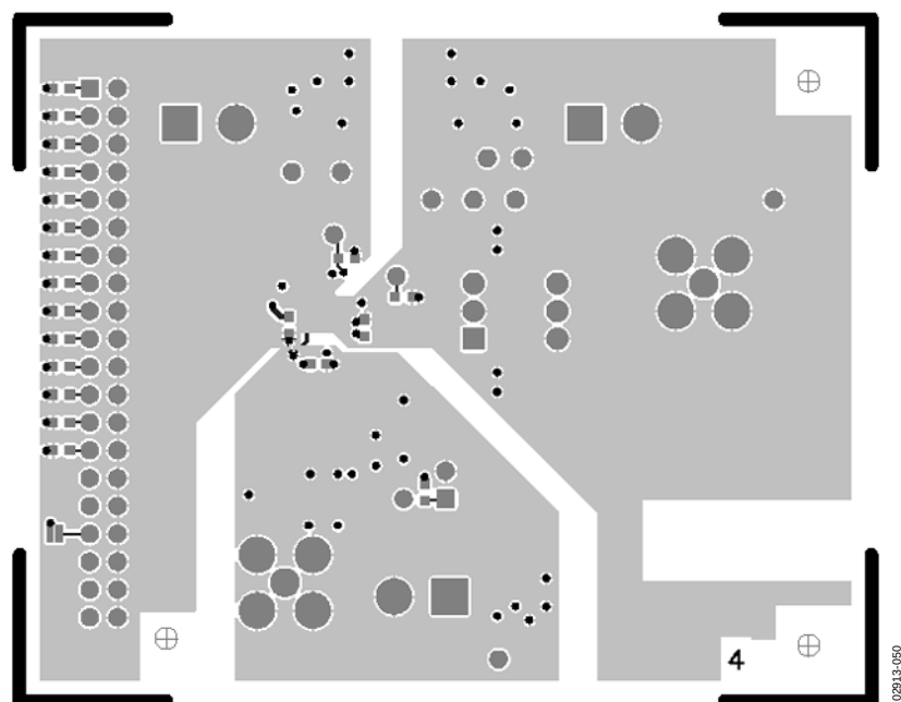
Figure 53. LFCSP Evaluation Board Layout—Secondary Side
