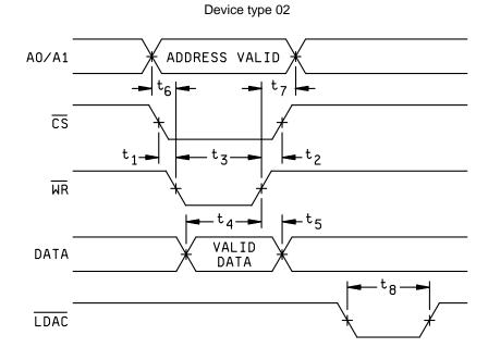
FIGURE 3. Timing waveforms.
