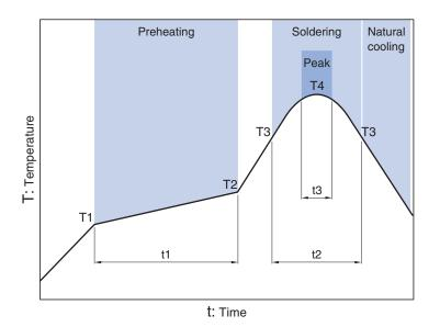
Preheating Soldering Peak Temp. Time Time Temp. Temp. Time T1 T2 t1 тз t2 Т4 t3 150°C 180°C 60 to 120s 230°C 30s 260°C 10s
