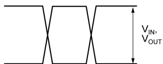
Figure 5a. Single-Ended Voltage Swing
