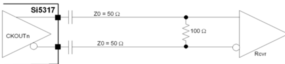
Figure 11. Typical Differential Output Circuit
