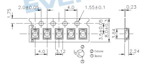
TOLERANCES UNLESS DIMENSION±0.1 ANGLE±0.5 UNIT:mm
