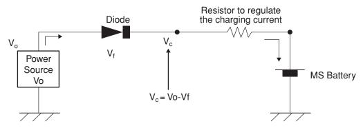
A resistor must be inserted to regulate the charging current, because our rechargeable batteries have a limit for charging current.
