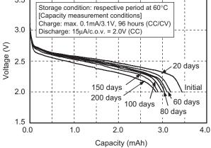
Floating Characteristics (60°C, applied voltage 3.1V)
