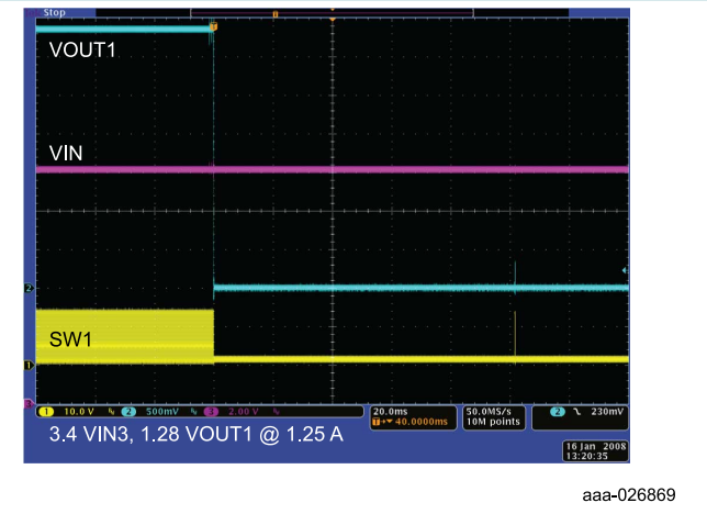
Figure 15. CH1 Short-circuit Response
