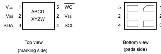
Figure 3. UFDFPN5 (DFN5) package connections
