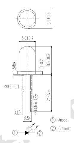
Note: Tolerances unless dimensions ±0.25mm
