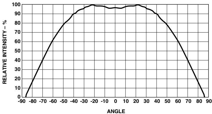
Figure 5b. Relative intensity vs. angle for HSMx-C177 and HSMx-C197.
