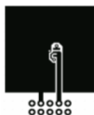
a) 78^\circ\text{C/W} when mounted on a 1 in 2 pad of 2 oz copper
