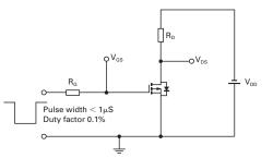
Switching time test circuit
