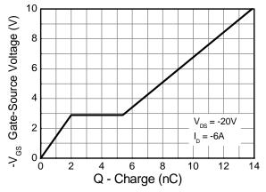
Gate-Source Voltage v Gate Charge
