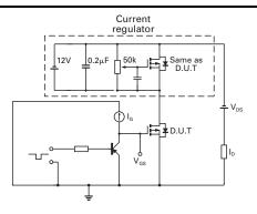
Gate charge test circuit
