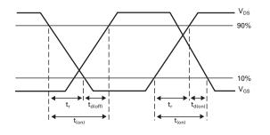
Switching time waveforms
