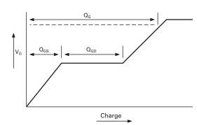
Basic gate charge waveform
