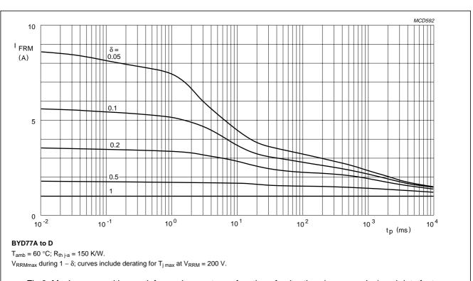
Fig.8 Maximum repetitive peak forward current as a function of pulse time (square pulse) and duty factor.
