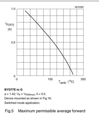
Fig.5 Maximum permissible average forward current as a function of ambient temperature (including losses due to reverse leakage).
