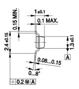
Note: Mold flash, protrusions or gate burrs of 0,2 mm max. per side are not included
