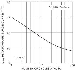
Fig. 5 Max Non-Repetitive Peak Forward Surge Current
