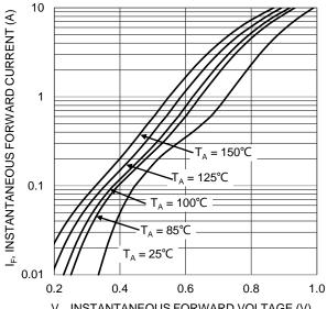
V<sub>F</sub>, INSTANTANEOUS FORWARD VOLTAGE (V) Fig.1 Typical Forward Characteristic
