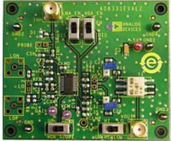
Figure 95. Photograph of AD8331-EVALZ
