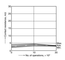
5-(3). Electrical life test (Lamp load) Sample: ACNM3112, 3pcs. Load: inrush: 84A/steady: 12A Operating frequency: ON 1s, OFF 14s Ambient temperature: Room temperature
