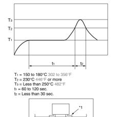
Temperature profile indicates the temperature of the soldered part (Note 1) of terminals on the surface of the PC board, however, for other areas such as the surface of relay case, make a setting so that you do not exceed the recommended conditions.
