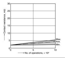
5-(2). Electrical life test (Motor load) Sample: ACNM7112, 3pcs.
