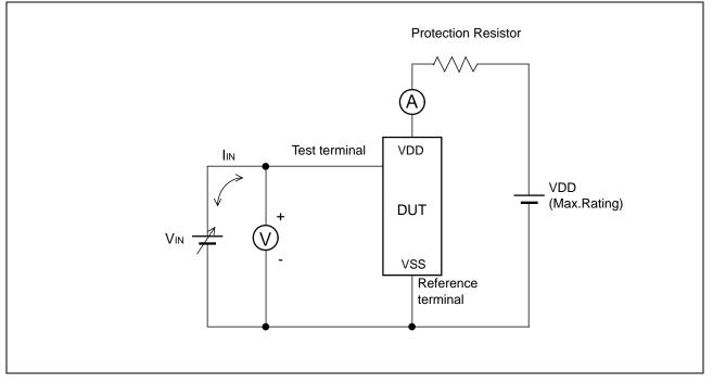
Note : The voltage V<sub>IN</sub> is increased gradually and the current I<sub>IN</sub> of 300 mA at maximum shall flow.
