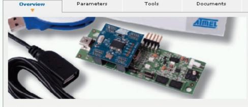
This fully integrated security module designed to be integrated into embedded systems. It is for TWI, I2C-compliant protocols and conforms to (TCG) v1.2 specifications.
