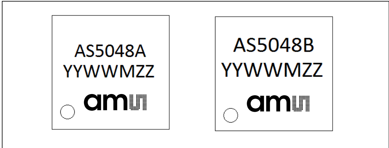
Figure 39: Package Markings for AS5048A & AS5048B
