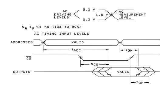
FIGURE 4. AC read timing diagram.
